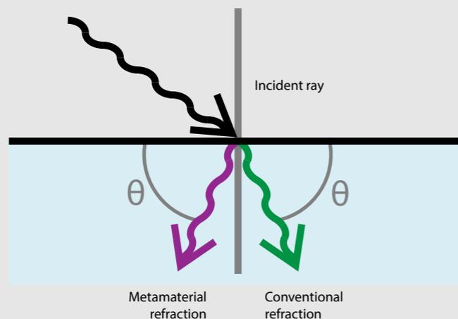
**Nature improved:** The green arrow shows the refracted path of a ray of light as it passes from air into a more dense medium like water or glass. Metamaterials can be specifically produced to give a negative refractive index
