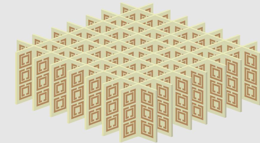
**Microscale:** Conventional electromagnetic metamaterials are made from sheets of fiberglass slotted together with exactly folded wires embedded to manipulate the wave as desired. Above is an array used on microwaves, with each copper square measuring less than 2mm across.
